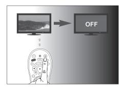
4 When the device is off, immediately press and release **OK** to save the code. The blue LED indicator will turn off.
