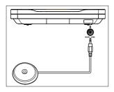
2 Place the calibration microphone as close to the seating position as possible, at ear height.
