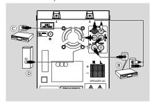
Using the VCR for recording DVDs (B) Connect one of the system's VIDEO OUT jacks to the corresponding VIDEO IN jack and LINE OUT (R/L) jacks to the AUDIO IN jacks on the VCR. This will allow you to make analogue stereo (two channel, right and left) recordings.
