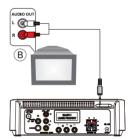
® To listen to TV through this system, use a cinch cable (not supplied) to connect AUX IN jack (3.5mm) to the corresponding AUDIO OUT jacks on the TV set.
