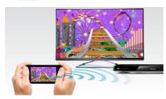
MiracastTM is a peer-to-peer wireless screencasting standard formed via Wi-Fi Direct connections. Simplified user interface like mirroring the portable device's screen to a bigger screen on a Miracast™ certified device, not limited by pre-built codecs for decoding.
