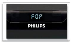
Digital Sound Control offers you a choice of pre-set Jazz, Rock, Pop and Classic controls you can use to optimise the frequency ranges for different musical styles. Each mode uses graphic equalizing technology to automatically adjust the sound balance and enhance the most important sound frequencies in your chosen music style. Ultimately, Digital Sound Control makes it easy for you get the most out of your music by precisely adjusting the sound balance to match the type of music you are playing.
