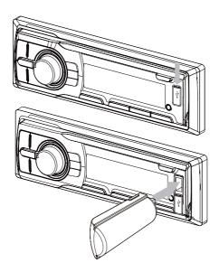
Insert the USB device into the USB socket.
