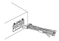
$\mathbf{2}$  Connect the other end of the supplied standard connector to the unit.
