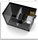
With its box-within-a-box design, this band pass subwoofer has two volume chambers to create more air capacity and deliver an altogether better bass sound with better balance and less distortion. The audio energy from the central driver is concentrated more effectively in the desired frequency output range, producing an overall sound image that is more focused and more accurately reproduced.
