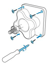
Insert the mounting screw on the bracket into the hole at the back of AW5000, then turn the rotating handle to tighten the screw.
