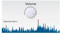
Anti-Clipping lets you play music louder and keeps it high quality, even when the battery is low. It accepts the input signals from 300mV to 1000mV and keeps your speakers safe from damage by distortion. This speaker handles anti-clipping through a dedicated audio limiter IC. This monitors the musical signal as it goes through the amplifier and keeps peaks within
