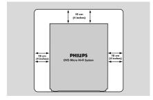
The ventilation should not be impeded by covering the ventilation openings with items, such as newspapers table-cloths, curtains, etc.
