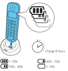
Flashing: low battery Scrolling: charging in progress
