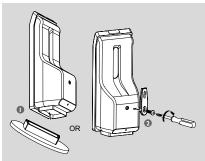
Before connecting the speakers to the DVD system, firmly attach the mini speaker stands to the surround speakers as shown in the above diagram.
