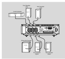
Connect the supplied speaker systems using the fixed speaker cables by matching the colors of the jacks and speaker cable connectors.
