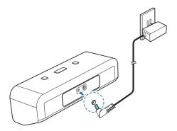
Connect the AC power adaptor, one end to the power socket on the back of the unit, and the other the wall power supply.
