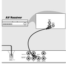
Receiver has a PCM, Dolby Digital, or MPEG2 decoder
