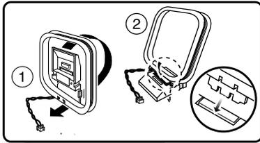
MW loop antenna
