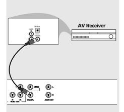
Receiver has a PCM, Dolby Digital, or MPEG2 decoder
