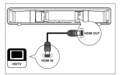
1 Connect a HDMI cable (supplied) from the HDMI OUT on this unit to the HDMI IN jack on your TV.
