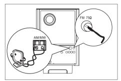
If you want to receive AM/MW radio band, connect the AM loop antenna (supplied) to the AM/MW jacks on this DVD Home Theater unit.
