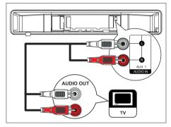
1 Connect an audio cable (not supplied) from the AUDIO IN-AUX1 jacks on this unit to the AUDIO OUT jacks on your TV.
