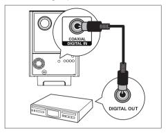
Connect a coaxial cable (not supplied) from the **DIGITAL IN-COAXIAL** jack on the subwoofer to the COAXIAL/DIGITAL OUT jack on the device.
