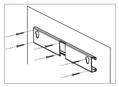
Hook the DVD Home Theater unit firmly onto the mounted bracket. Slide the knobs through the key holes and lock into position.
