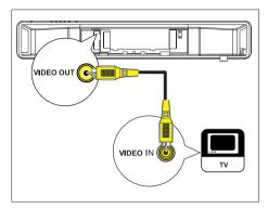
Connect a composite video cable (supplied) from the VIDEO OUT jack on this unit to the video input jack on your TV.
