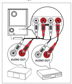
Connect an audio cable (not supplied) from the AUDIO IN-AUX2 or AUX3 jacks on the subwoofer to the AUDIO OUT jacks on the device.
