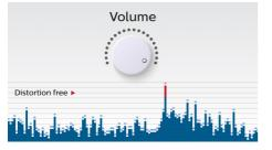
Anti-Clipping lets you play music louder and keeps the quality high, even when the battery is low. It accepts input signals from 300 mV to 1000 mV and keeps your speakers safe from damage by distortion. This speaker handles anti-clipping through a dedicated audio limiter IC. This monitors the musical signal as it goes through the amplifier and keeps
