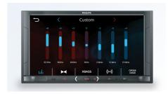
7-band parametric equalizer with 8 presets
