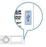
Insert the USB device into the USB socket.
