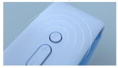
One long press of the play/pause button gets this wireless Bluetooth speaker ready to pair. Once paired, the speaker remembers the last device it was paired with. Wireless range of the speaker is 10 m.
