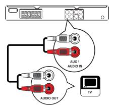
Connect the audio cables (not supplied) to the AUDIO IN-AUX1 jacks on this Home Theater System and the AUDIO output jacks on the TV.
