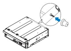
5 Install the sleeve into the dashboard and bend the tabs outwards to fix the sleeve. Slide the unit into the dashboard until you hear a click.
