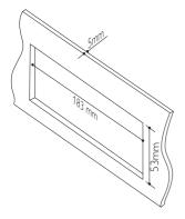
3 Install the sleeve into the dashboard and bend the tabs outward to fix the sleeve.
