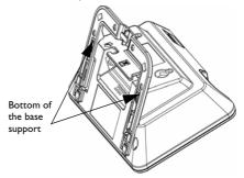
To remove, simply pull the base support away from the base unit.
