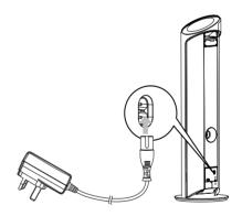
2 Connect the power plug to the wall outlet.
