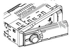
**3** Press the right side of the panel until it is locked into place.
