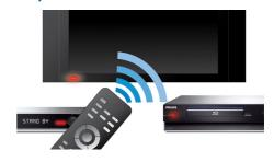
EasyLink lets you control multiple devices like DVD players, Blu-ray players, soundbar speakers, home cinema systems and TVs with one remote. It uses HDMI CEC industry-standard protocol to share functionality between devices through the HDMI cable. With one touch of a button, you can operate all your connected HDMI CEC enabled equipment simultaneously. Functions like standby and play can now be carried out with absolute ease.
