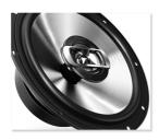
Inside the speaker, a diaphragm sits on top of a voice coil to produce a signal waveform once an input signal is received. It transforms the signal wave into a sound wave. Polypropylene is one of the lightest plastics ever invented and is great material for speaker diaphragms due to its weight, high strength, stiffness and tolerance for high temperatures. These polypropylene cones deliver high quality music by reacting to even the smallest sound signal to produce clear, vivid sound.
