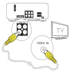
1 Connect the supplied composite video cable to:
