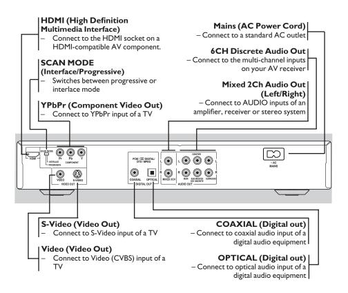
Caution: Do not touch the inner pins of the jacks on the rear panel. Electrostatis discharge may cause permanent damage to the system.
