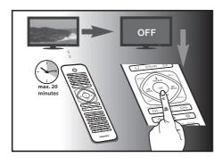
Operate the device with the universal remote. If your device responds correctly, it means you have saved the right code.
