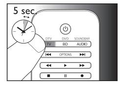
Point at your device with the universal remote. Then press and release **ψ** to start searching the code for your brand. A different infrared signal is sent every 2 seconds as the universal remote searches, indicated by a red flash.
