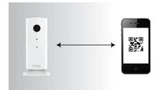
Quick and easy set-up allows you to pair the InSight wireless home monitor with an iPhone or iPad. Place the QR code image in front of the monitor lens to activate the InSight app. The monitor is ready to use when light turns solid green.
