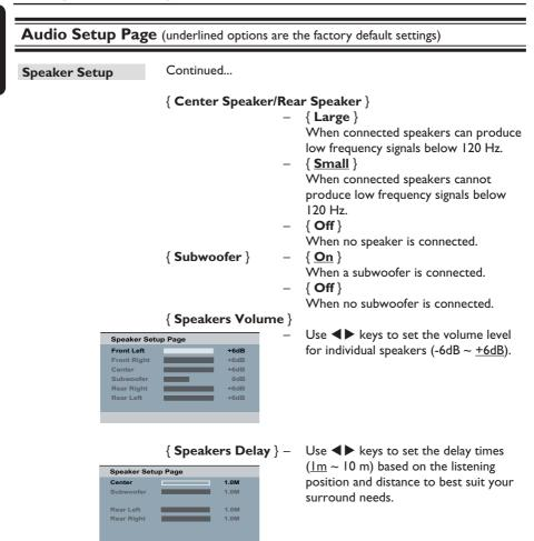
**Note:** Use the longer delay time settings when the rear speakers are closer to the listener than the front speakers.
