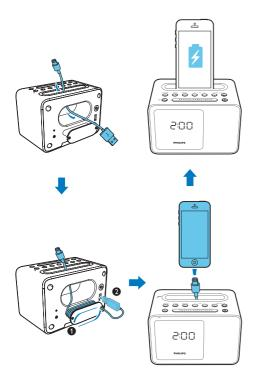
2 Connect the clock radio to AC power. → The phone begins to charge.
