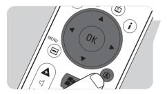
2 Use the remote control navigation keys (◄ ► ▲ ▼ - 6) to select the program you want to delete and press the OK key (19).
