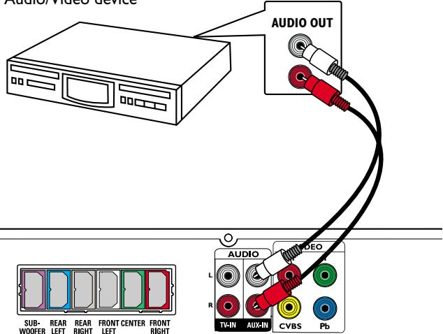
**Note:** Connect the **AUDIO OUTPUT** of other audio/video device to this DVD system in order to use the Home Theatre Audio System's surround sound capabilities. Press **AUX/DI** on the remote control in order to listen to the playback.
