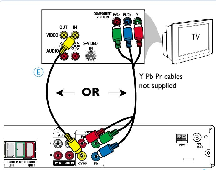
**Note:** For connecting to a Progressive Scan TV, refer to the user manual for proper connections and detailed set up.
