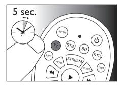
Point at your device with the universal remote. Then press and release U to start searching the code for your brand. A different infrared signal is sent every 2 seconds as the universal remote searches, indicated by a blue flash.
