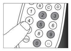
5 If the light is off, a valid code is saved. Otherwise, the light will flash once, and then remains on for code re-entry.
