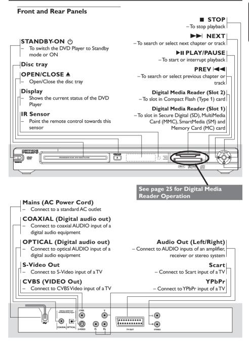
Caution: Do not touch the inner pins of the jacks on the rear panel. Electrostatic discharge may cause permanent damage to the unit.
