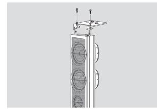
Attach a supplied speaker stand firmly to the bottom of each rear speaker using the supplied screws.
