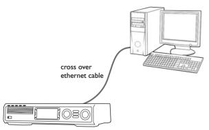
1 Connect ETHERNET on the Streamium System to the ethernet jack of the PC with a cross over ethernet cable (not supplied).
