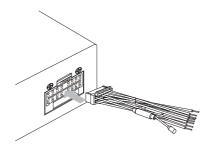
2 Connect the other end of the supplied standard connector to the unit.
