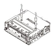
3 Remove the mounting sleeve with the supplied disassembly tools.
