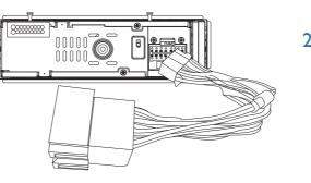
2 Connect the other end of supplied standard connector to the unit.
