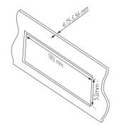
Ensure that car dashboard opening is within these measurements.
