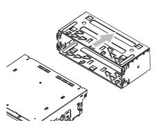
5 Install the sleeve into the dashboard and bend the tabs outward to fix the sleeve.
