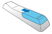
2 Insert 2 AAA batteries with correct polarity (+/-) as indicated.
