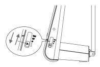
3 Turn the TV or FM radio to the desired channel/station. Move the dipoles in different directions up and down until the reception is achieved.
