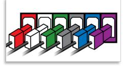
Color-coded connectors provide a simple and user-friendly solution to connect the speakers and subwoofer to the center unit of the home entertainment system simply by plugging the connectors in the matching colored interface at the rear of the center unit.
