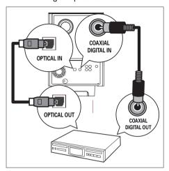
Connect a coaxial cable (not supplied) from the **DIGITAL IN-COAXIAL** socket on the subwoofer to the COAXIAL/ DIGITAL OUT socket on the device.
