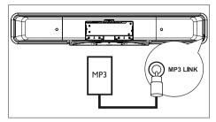
Connect a 3.5mm stereo audio cable (supplied) from the MP3 LINK socket on this unit to the phone socket on your portable media player (such as MP3 player).
