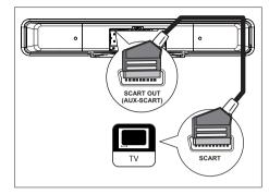
1 Connect a scart cable (supplied) from the SCART OUT (AUX-SCART) socket on this unit to the scart input socket on your TV.
