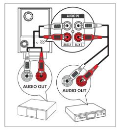
1 Connect an audio cable (not supplied) from the AUDIO IN-AUX2 or AUX3 sockets on the subwoofer to the AUDIO OUT sockets on the device.
