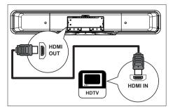
1 Connect a HDMI cable (supplied) from the HDMI OUT on this unit to the HDMI IN socket on your TV.
