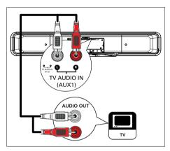
1 Connect an audio cable (not supplied) from the TV AUDIO IN (AUX1) sockets on this unit to the AUDIO OUT sockets on your TV.
