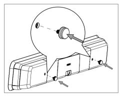
4 Position the supplied bracket on the wall, drill the screw holes and insert the rubber wall plugs (not supplied) into the holes.
