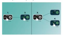
No router, no password, no apps needed for set up. Just long press the "GROUP" button on two speakers to set up for the first time. Repeat to add a 3rd, 4th, or 5th speaker. Each long press of the "Group" button adds one new speaker at a time. Multiroom music has never been easier. Once complete, the izzylink  $\ensuremath{^{\text{TM}}}$  network will be stored even when the speaker is unplugged.
