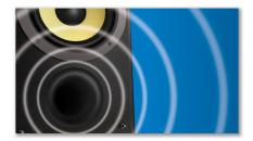
Bass Reflex Speaker System delivers a deep bass experience from a compact loudspeaker box system. It differs from a conventional loudspeaker box system in the addition of a bass pipe that is acoustically aligned to the woofer to optimize the low frequency roll-off of the system. The result is deeper controlled bass and lower distortion. The system works by resonating the air mass in the bass pipe to
